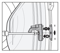
If you use too many spacers the door will not provide a sufficient seal when shut properly.
